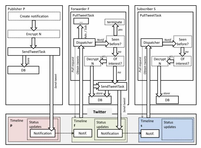
**Figure 3.1:** Information flow of a notification. The notification is created, encrypted and posted to the publisher's timeline. The notification is then picked up by a forwarder who follows the publisher. Next, the status update is being processed and finally posted on the forwarder's timeline. Lastly, the subscriber who follows the forwarder receives the notification. [8]
