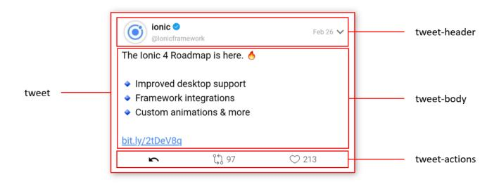
**Figure 5.2:** Composition of the tweet component from three other components. Several tweet components are in turn combined to form a feed component.
