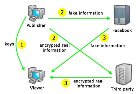
**Figure 3.2:** Schematic representation of the Setup Phase (1), Encryption Phase (2) and Decryption Phase (3) and the data flow taking place between the entities.
