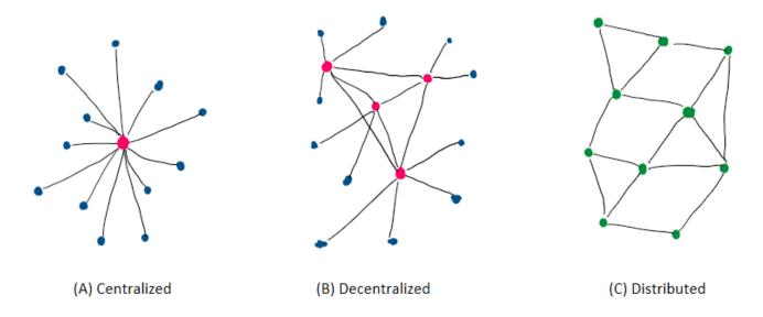
Figure 2.1: Schematic representation of various software system architectures. In centralized applications (A), all clients (blue) are in connection with a central server (red), while in decentralized applications (B) several servers provide for improved stability. In distributed applications (C), all nodes have the same role with the same tasks, which is why we also speak of peers (green).
