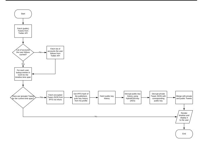
Figure 5.5: Flow chart of the process for loading the home timeline for a user
