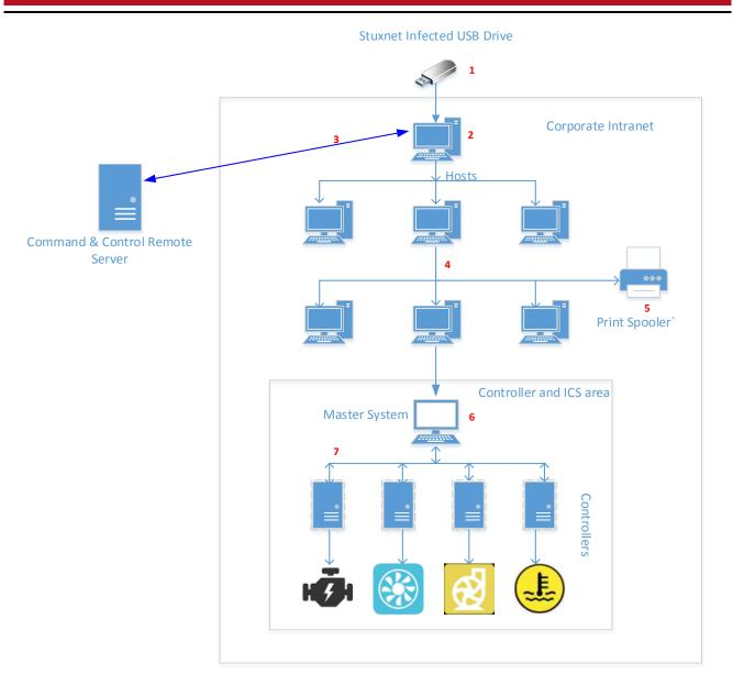
Figure 14: Stuxnet Architecture
