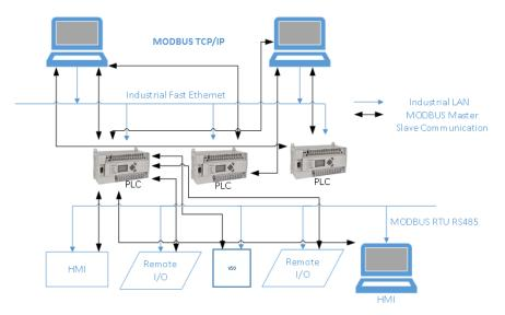
Figure 12: SCADA Master and Slave profile
