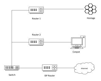
Figure 21: Conpot and HosTaGe environment setup
