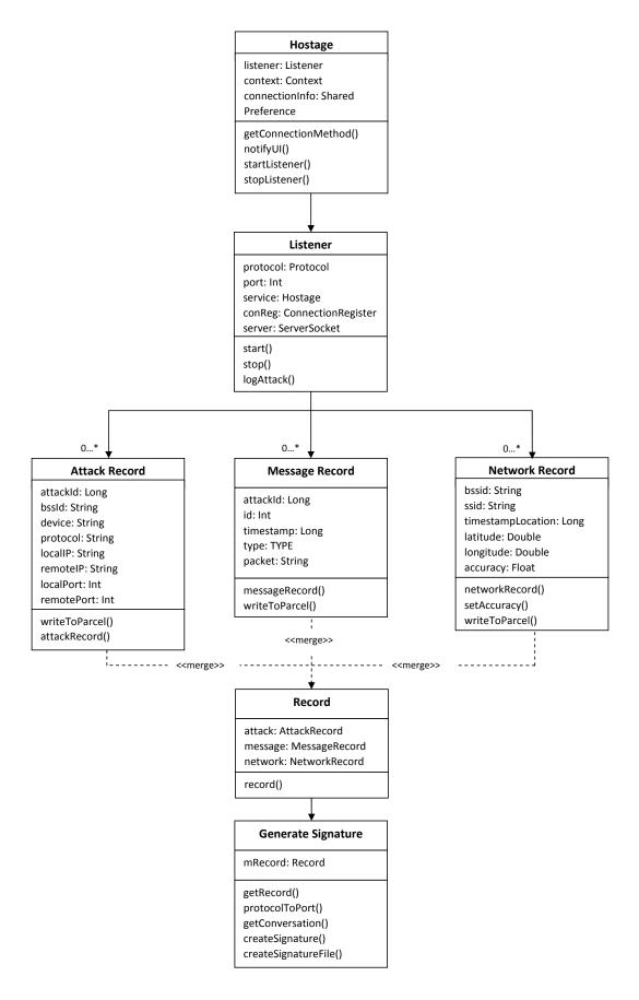
Figure 20: Signature Generator Class Diagram
