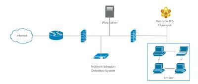
Figure 11: Network Architecture of IDS and HosTaGe
