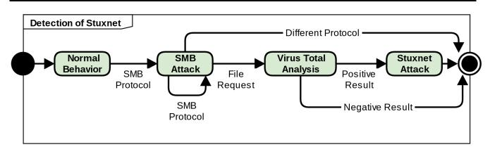
Figure 10: EFSM for PLD in the case of Stuxnet propagation [13]
