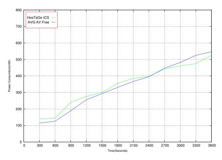
Figure 31: HosTaGe ICS Power Consumption in comparison with AVG
