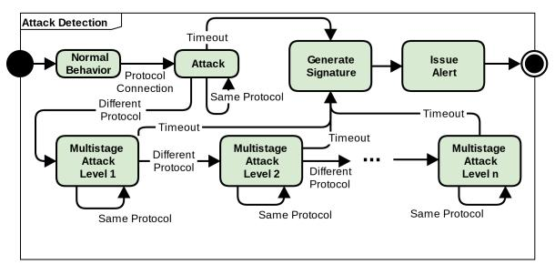
Figure 9: EFSM of the attack detection and signature generation mechanism [13]
